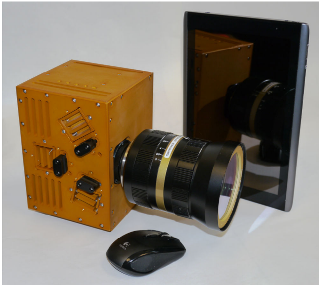
Optional tablet to control camera and embedded computer
